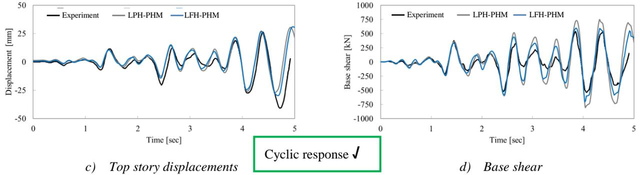
Figure 4. Experimental vs. numerical results of the RC frame with infill walls for model: LFH-PHM & LPH-PHM.
