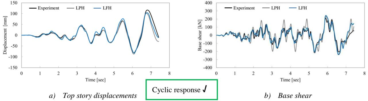
Figure 3. Comparison of the experimental results and numerical prediction of the RC bare frame for models LFH & LPH.
