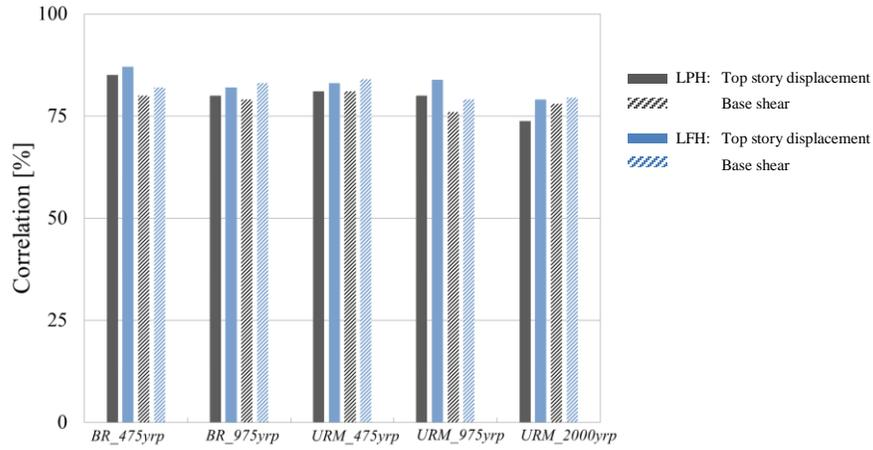
Figure 5. Correlation between experimental and numerical displacement time histories of models LPH & LFH for the bare frame (BR) and the models LPH-PHM & LFH-PHM for the frame with infill walls (URM) for different intensity levels.
