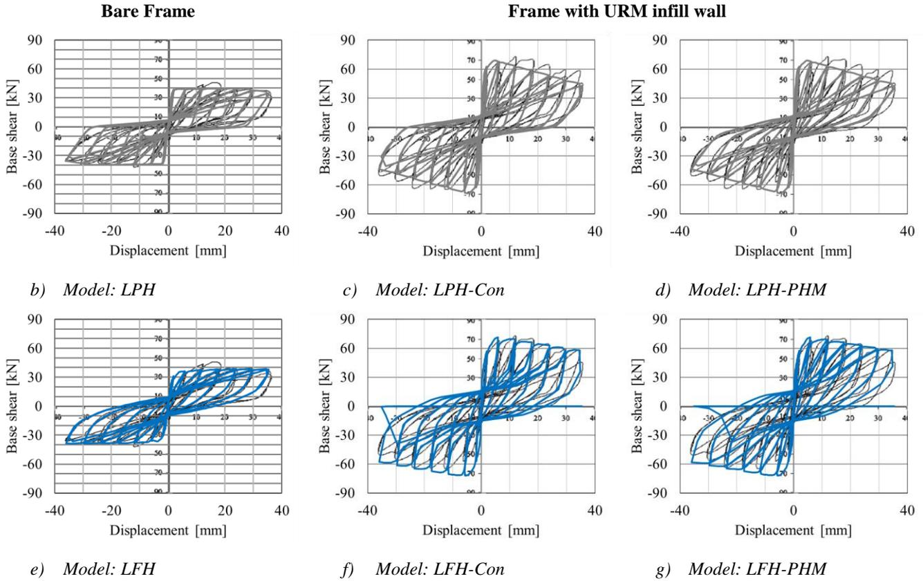
Figure 2. Comparison of the hysteretic experimental (black line) and numerical (LPH ... grey line, LFH ... blue line) results for the different model combinations [Note: Comparison mainly done graphically via digitalization of published results.]
