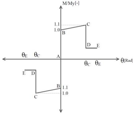
a) Moment plastic hinge model for beams
